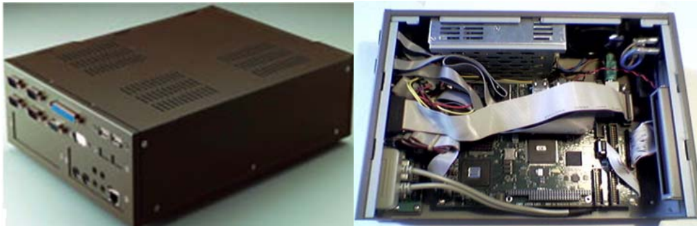
Fig. 3. Micro-PC is installed in Micro-BOX
