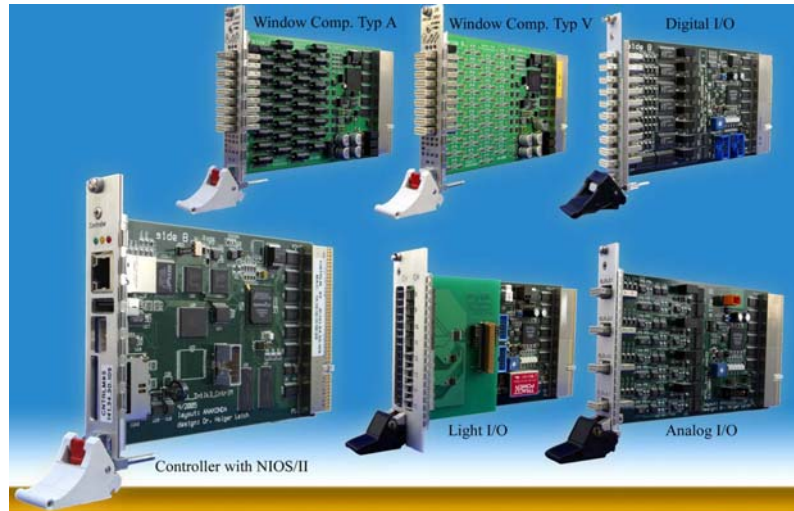
Fig. 5. Interlock Controller & Slave Modules
