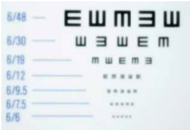
Figure 12. Snapshot taken with digital camera Nikon D70S attached with a pinhole with d = 0,26 mm (near optimal pinhole). Resolution reaches line 5
