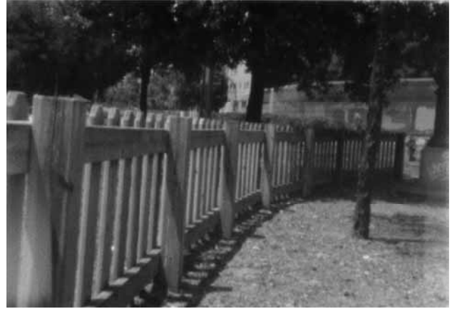
Figure 4. Snapshot taken with 135 mm analog pinhole camera to show soft focus and large depth of field
