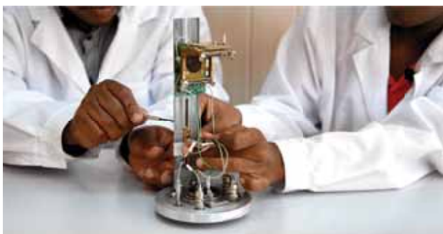
Figure 10. Assembling of the detection system of the light ion spectrometer
