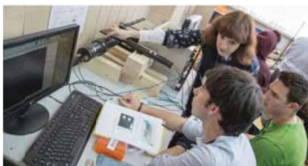
Figure 8. Work with the scintillation telescope of cosmic rays
