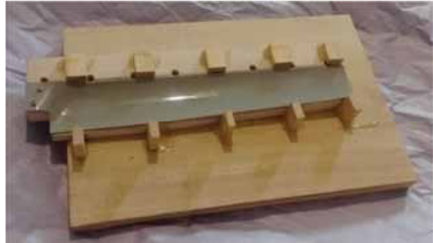
Figure 9. The shape of the modern wind turbine basically is formed after the PVC plate gradually cools and hardens
