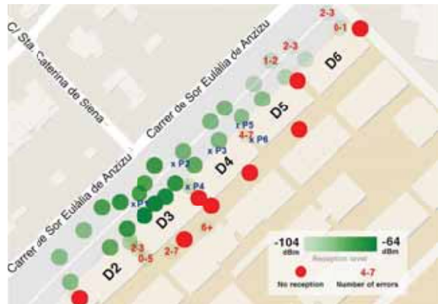
Figure 9. WiFi link performance map. (Green dots) Received signal strength [dBm] (Yagi antenna lab team). (Red dots) Points without reception (Yagi). (Blue points P1-P6) “Patch antenna” team measurement points. (Adapted from M. Oller, J.A. Ballester and C. Segarra, FDR, spring 2016)
