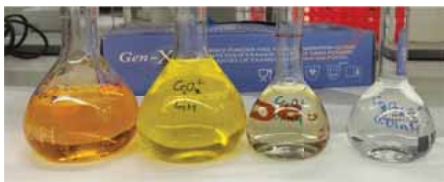
Figure 2. Ammonium dichromate solutions. From left to right, 10mM 1mM 0.1mM 0.01mM. The more concentrated the dichromate solution is, the more colourful it is
