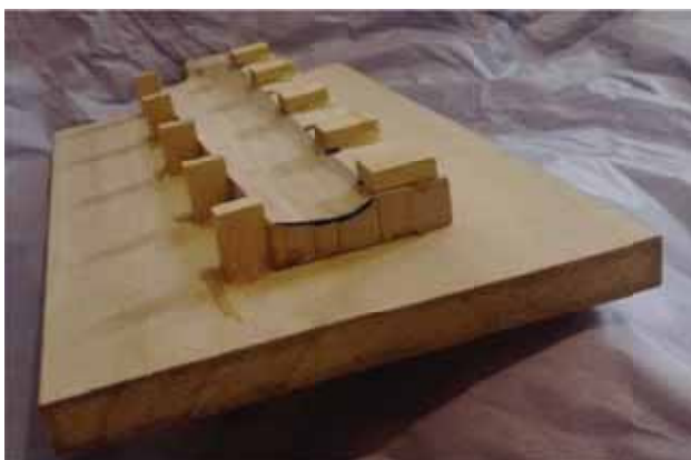
Figure 5.b. The mold regulates the curved surface of the wind-turbine
