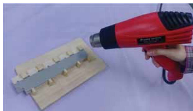
Figure 7. Heat the PVC plate on the mold with a hot air gun. The tool that looks like a hair dryer is a hot air gun
