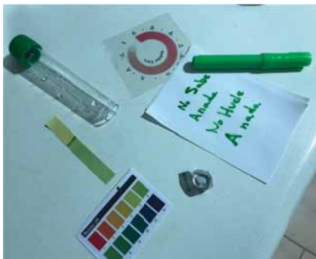
Figure 3. The kit provided to students allows to analyze drinking water
