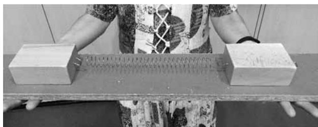
Figure 11. The blocks on the board with sandpaper connected with the spring
