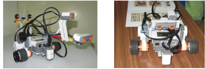
Figure 3. Two robots with the ultrasonic sensor on different locations
