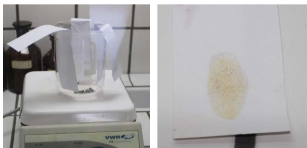
Figure 3. Revealing latent fingerprints using iodine fuming
