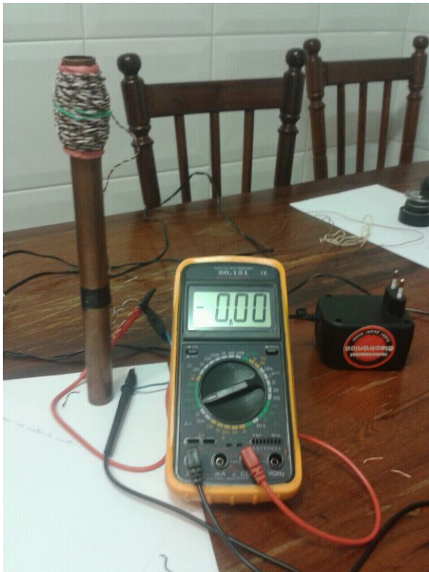
Figure 1. Main set-up: copper tube with a coil of wire coiled around a PVC pipe
