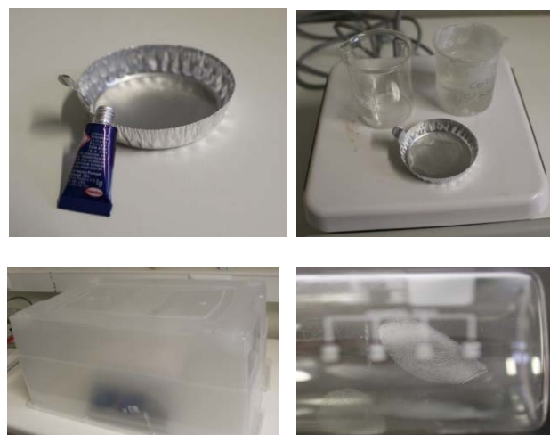
Figure 2. Revealing latent fingerprints using superglue fuming
