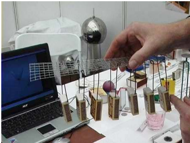
Figure 4. Wave machine made from match boxes
