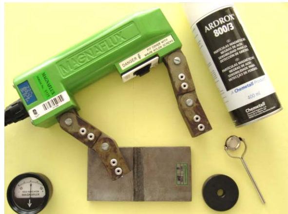
Figure 10. Equipment necessary to illustrate the magnetic particle inspection
