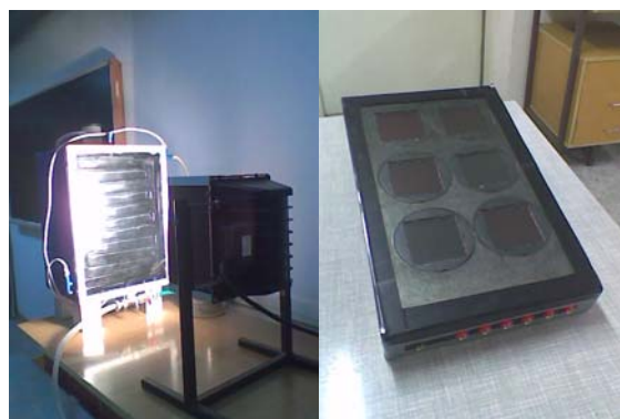
Figure 8. Transformation of solar energy: left - flat plate solar collector; right - a photovoltaic module made of solar cells of garden lamps
