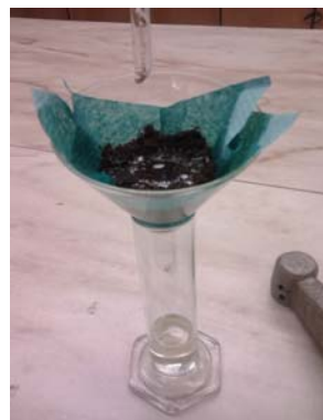
Figure 3. Collecting drops of water passing through the soil
