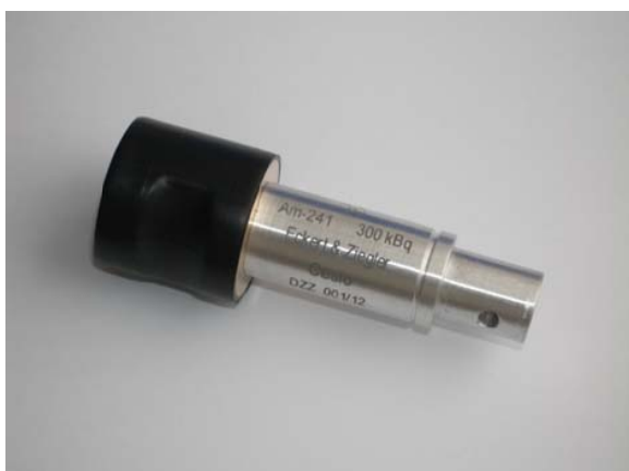
Figure 4. Demonstration gamma radiation source DZZ Gama 300 kBq
