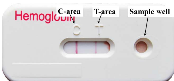
Figure 5. SERATEC® test – used. C area is a control area (colour change shows that the chromatography was successful), T area is testing area (colour change shows that the human haemoglobin is present) and sample well are shown (for droplets dropping).
